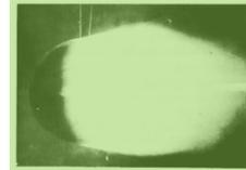
Fig. 2.20. Flow past a sphere at a subcritical Reynolds number; from Wisselsberger [22]
