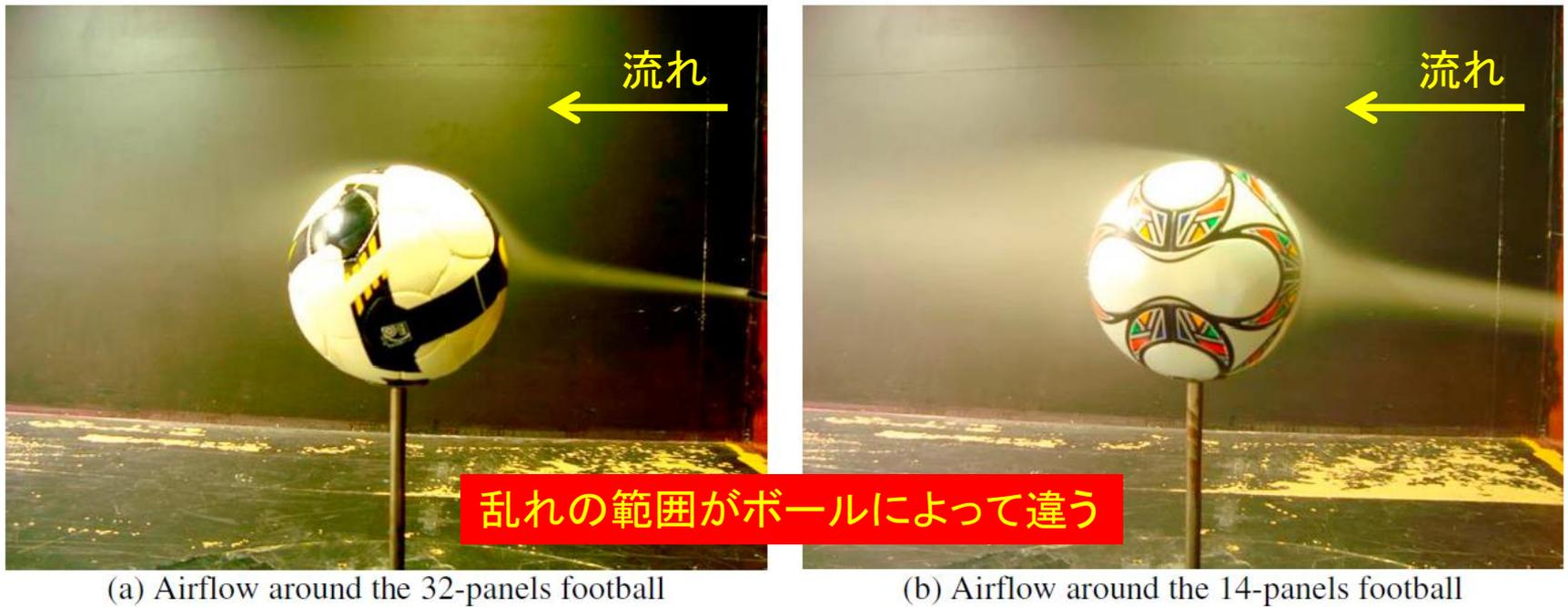
Fig. 3. Airflow structure of football with smoke flow visualization
